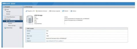
We have managed to add the USB-Disk as VMFS Datstore and we can now deploy VMs on it. I will proceed with the installation of vCenter Appliance.
